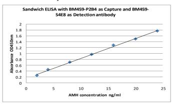
An example of a sandwich ELISA using sera evaluated by Roche reagent with chemiluminescence using BM459-P2B4 as the Capture antibody and BM459-S4E8 as the Detection antibody.
